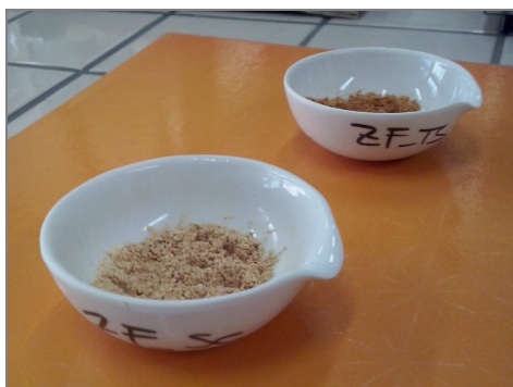
Figure 1. Fresh ZnFe_2O_4/SBA-15 sorbents through two-solvents- (top) and self-combustion-impregnation (bottom).
