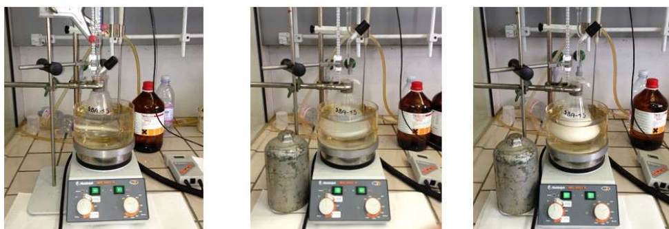
Figure 2. Evolution of the SBA-15 preparation before (left), during (centre), and after (right) the addition of tetraethyl ortho silicate.
